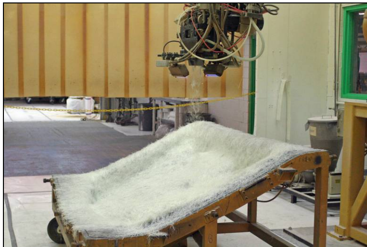
RimFire™ application of fiberglass reinforcement to the mold cavity
