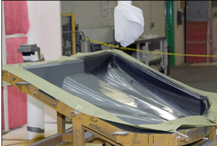
Robotic application of the in-mold coating to the mold surface
