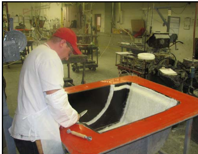
Glass Reinforcement Placement in Light Resin Transfer Mold (LRTM)
