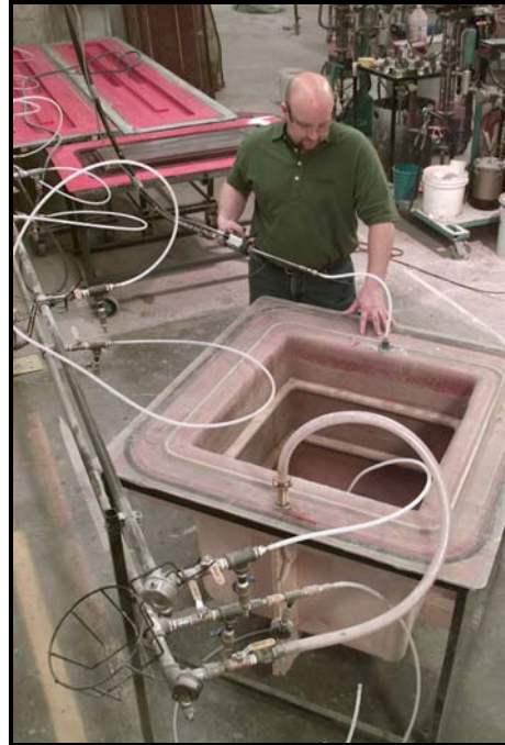
Light Resin Transfer Molding (LRTM) Process
