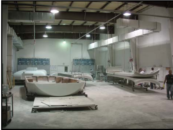
Nacelle components in queue for trim and assembly
